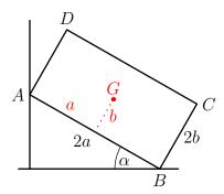
It is now clear that the distance of G from the wall is  $a\cos\alpha$  (horizontal distance from wall to midpoint of AB) plus  $b\sin\alpha$  (horizontal distance from midpoint of AB to G), so a total of  $a\cos\alpha + b\sin\alpha$ .
