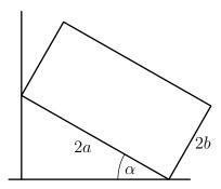
The diagram shows a uniform rectangular lamina with sides of lengths 2a and 2b leaning against a rough vertical wall, with one corner resting on a rough horizontal plane. The plane of the lamina is vertical and perpendicular to the wall, and one edge makes an angle of  $\alpha$  with the horizontal plane. Show that the centre of mass of the lamina is a distance  $a \cos \alpha + b \sin \alpha$  from the wall.
